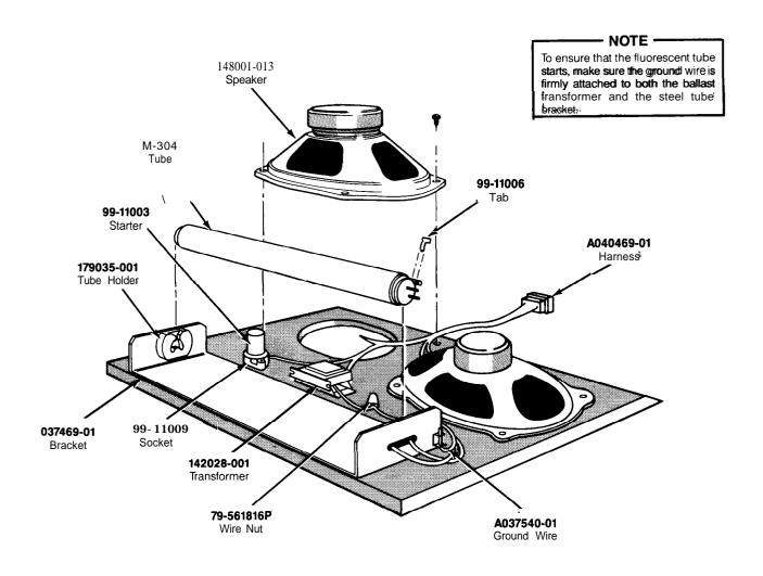
Figure 5-4 Fluorescent Tube and Speaker Assembly A040383-01 A
