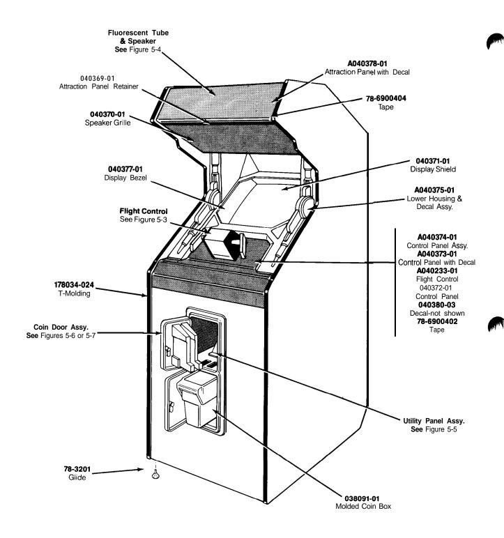
Figure 5-1A Cabinet-Mounted Assemblies US-Built Cabinet A040344-01 A
