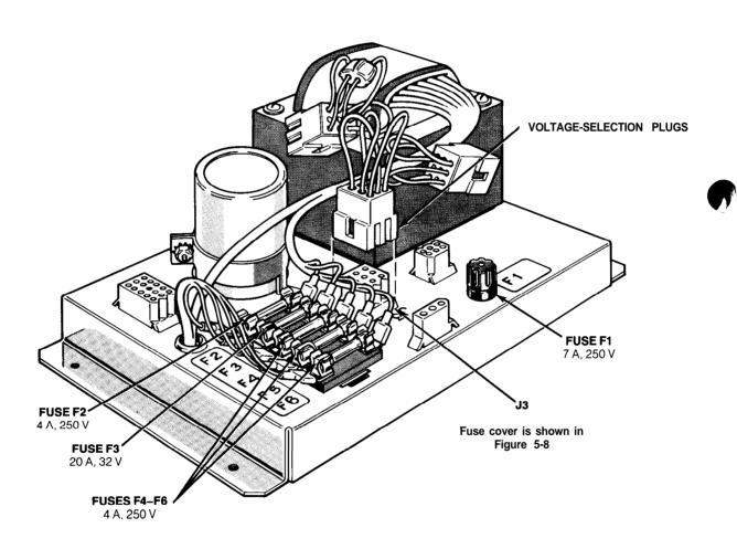
Figure 1-2 Voltage-Selection Plug and Fuse Locations
