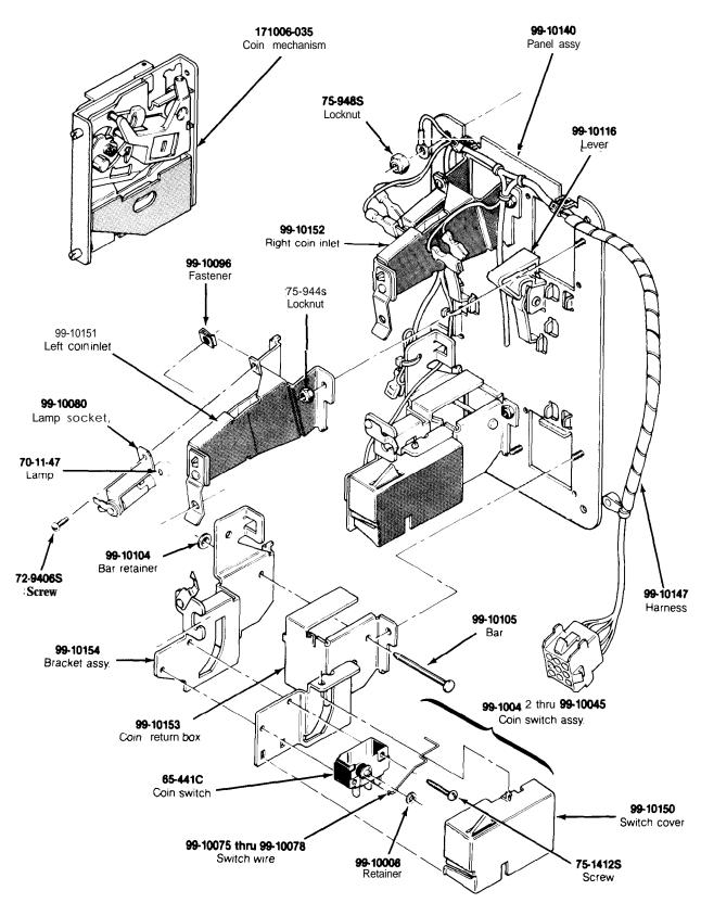
Figure 5-7 American-Made Coin-Door Assembly 171027-001 A
