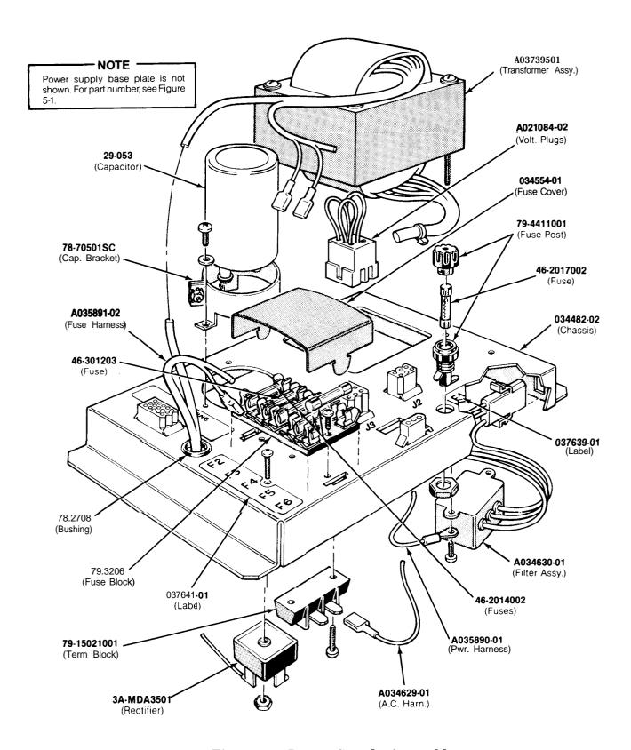
Figure 5-8 Power Supply Assembly A037396-04 F
