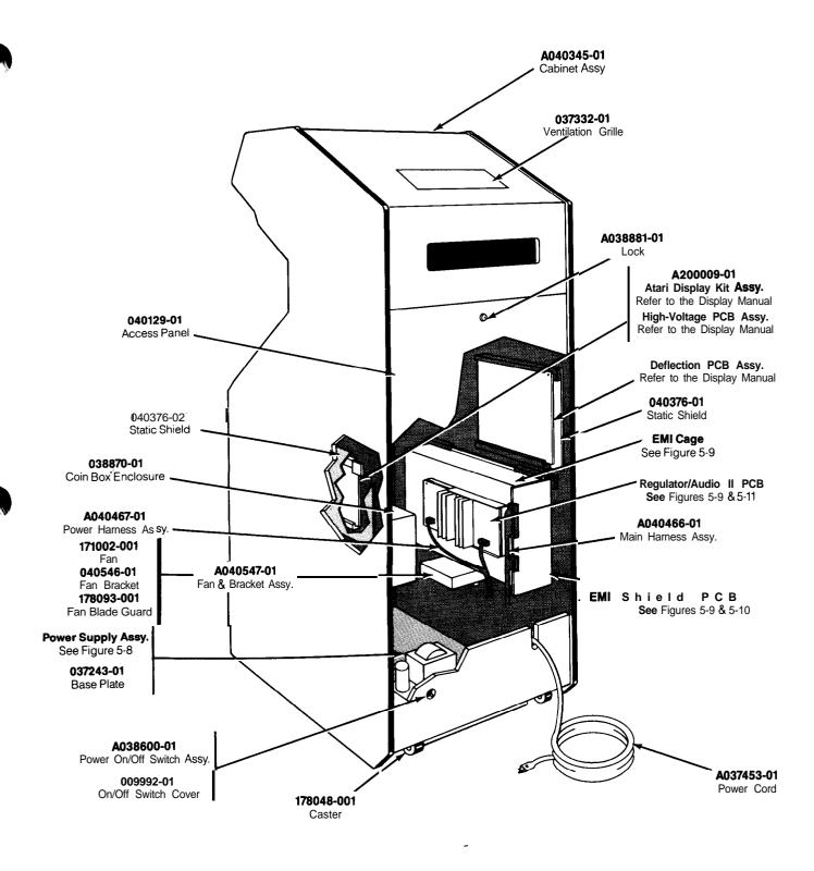
Figure 5-1A Cabinet-Mounted Assemblies, continued US-Built Cabinet A040344-01 A
