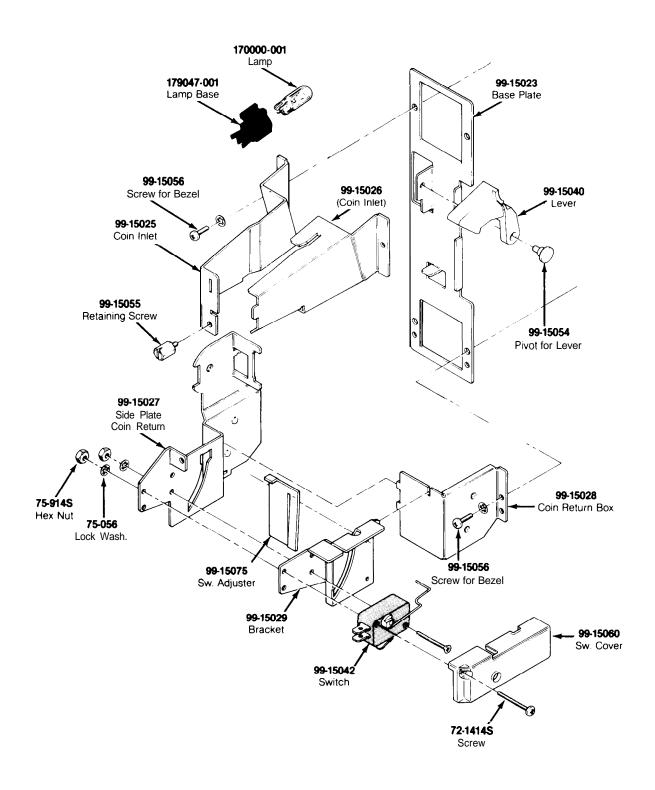
Figure 5-6 Vertically Mounted Coin Door 171034-xxx A
