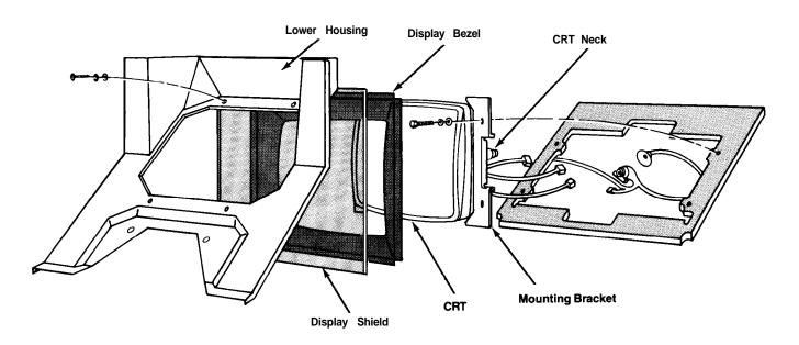
Figure 4-3 Removing the CRT Assembly
