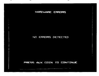
Figure 2-3 Hardware Errors Display-Test Passes
