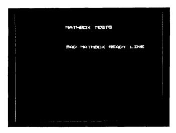
Figure 2-7 Mathbox Tests Display-Test Fails
