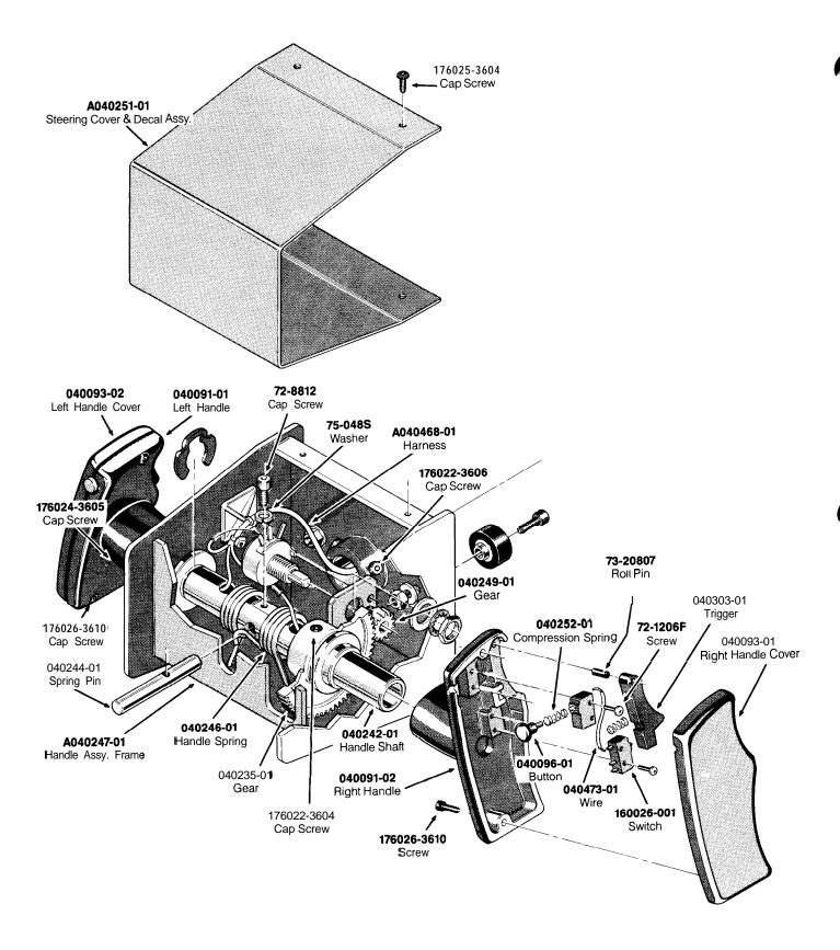
Figure 5-3 Flight Control Assembly A040233-01 A
