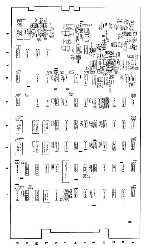
Figure 5-13 Analog Vector-Generator (AVG) PCB Assembly A038463-21 A
