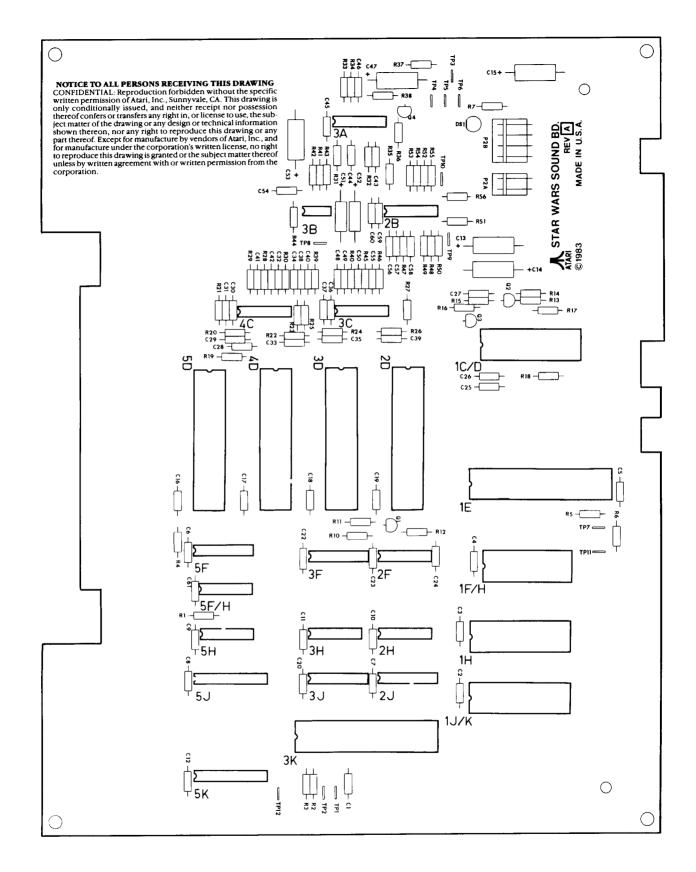
Figure 5-14 Sound PCB Assembly, A040260-01 A
