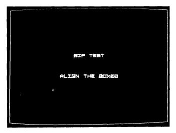
Figure 2-11 Bipolar Offset Test Display-Test Passes
