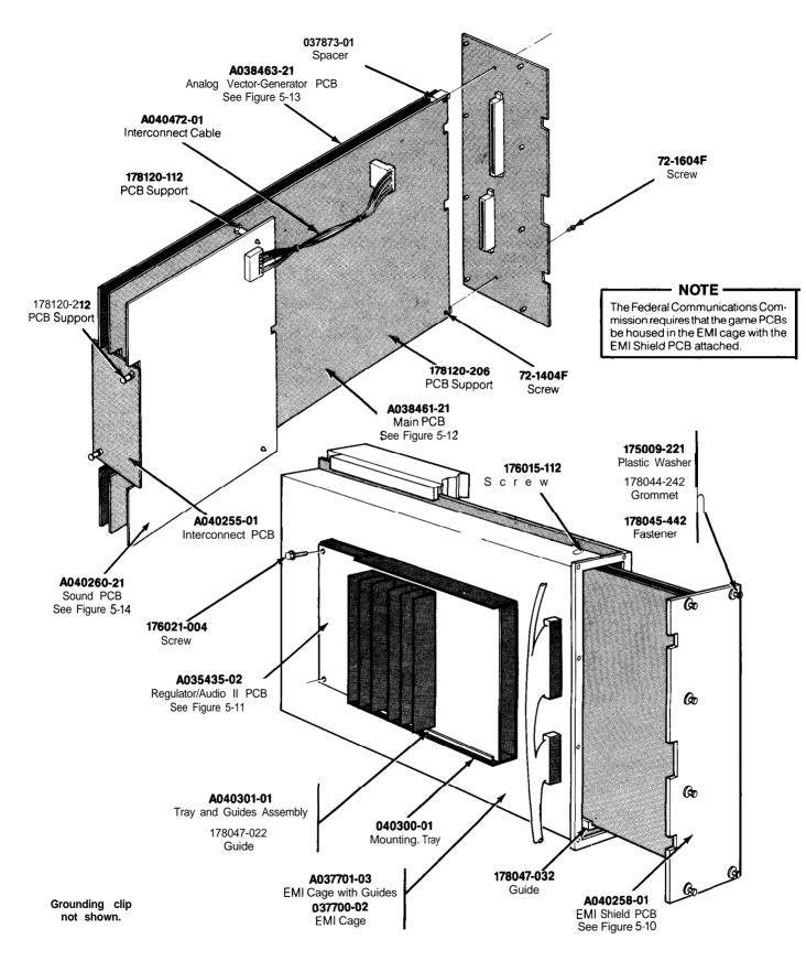
Figure 5-9A PCB Mounting Hardware US-Built Cabinet
