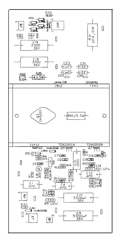
Figure 5-11 Regulator/Audio II PCB Assembly A035435-02 G
