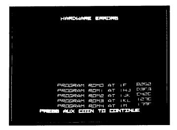
Figure 2-4 Hardware Errors Display-Test Fails
