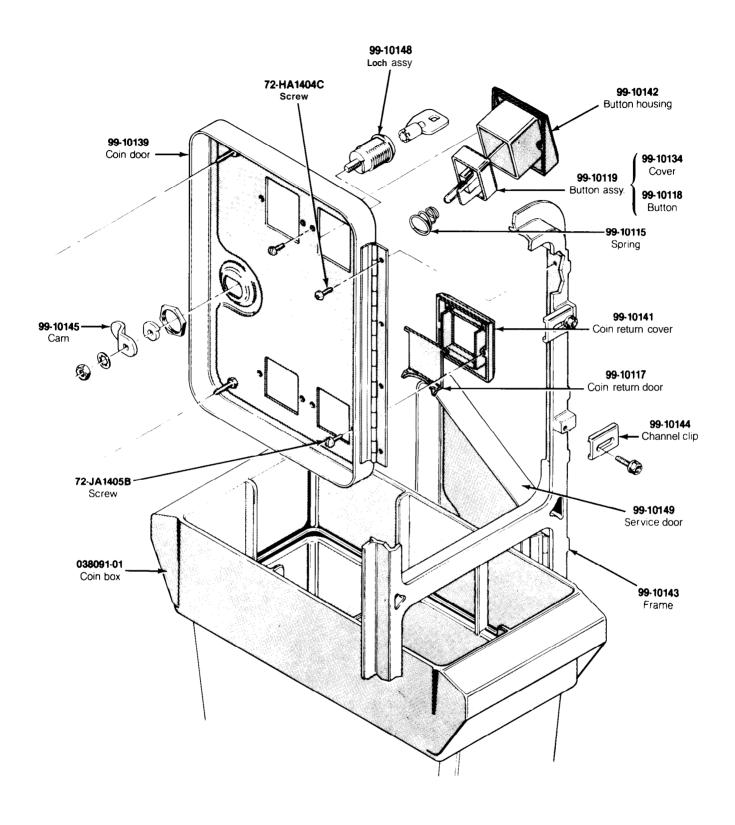
Figure 5-7 American-Made Coin-Door Assembly, continued 17102 7-001 A
