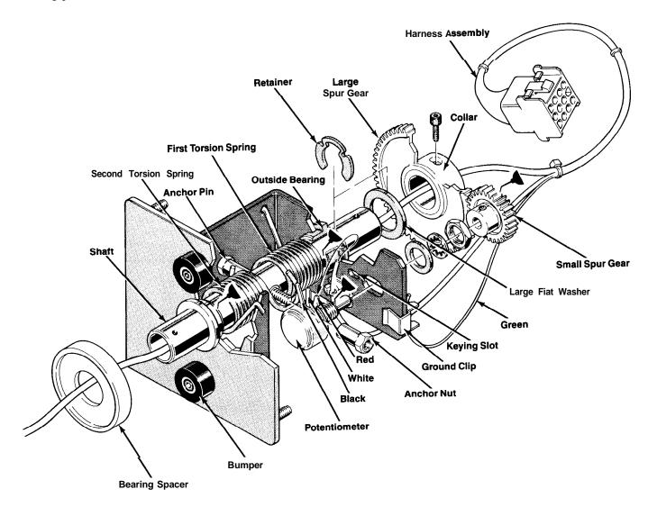
Figure 4-2 Steering Assembly
